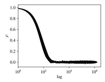
**Fig. A.1.** Autocorrelation functions for the 26 parameters of the elliptical model, the log likelihood, and log posterior, computed on the last 1,500,000 steps of the Metropolis algorithm. The maximum integrated autocorrelation time is 223, which corresponds to an effective sample size of 6,721.
