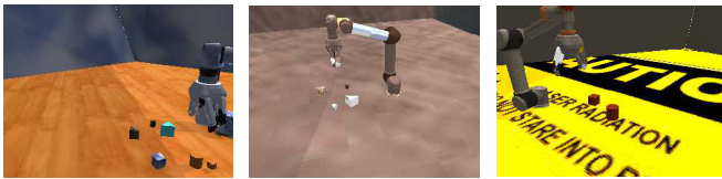
Fig. 4: Examples of synthetic training images. We generate images displaying the robot and a variable number of objects in its workspace. The images are taken by cameras with different viewpoints and depicting large scene appearance variations.
