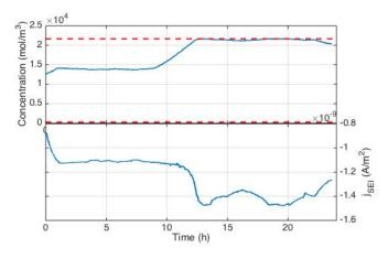
Figure 6. **Top:** Profile of the ion concentration at the anode particle surface (blue line) and its boundaries (red dashed lines). **Bottom:** Profile of the current density of the parasitic reaction leading to SEI formation.
