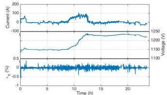
Figure 5. **Top:** BESS current profile simulated through the detailed electrochemical model. **Middle:** BESS simulated voltage profile. **Bottom:** One-stepahead prediction error of the voltage predicted through the SPM.
