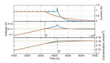
Figure 3. Battery charge with a fixed power set-point. **Top:** cell current, **middle:** cell voltage, **bottom:** anode surface ion concentration. Red lines refer to an MPC based on I-V limits, blue lines refer to a physics-based MPC. Yellow dashed lines in the middle and bottom plots represent the tresholds for the voltage and anode concentration respectively.
