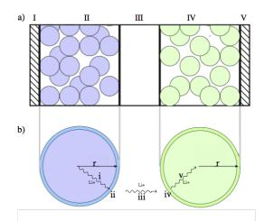
Figure 2. a) Structure of a Li-ion cell: I) negative current collector; II) anode; III) separator; IV) cathode; V) positive current collector. b) Single particle model schematic.
