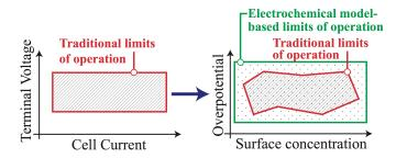
Figure 1. Qualitative comparison of the traditional operational constraints for a Li-ion cell, based on measurable quantities (left) and allowed by the knowledge of actual cell physical states (right) [4].
