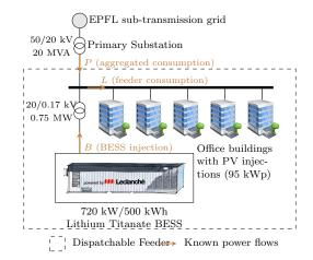
Fig. 2. The dispatchable feeder configuration (Sossan et al. (2016)).
