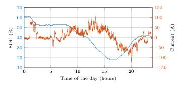
Fig. 7. Measured BESS SOC and DC current on 13/01/2016.
