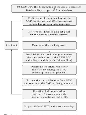
Fig. 4. Flow chart showing real-time operation during 24 hours.
