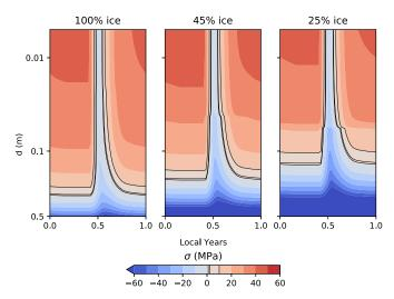
**Fig. 10.** Thermal stress for a latitude of  $-60^{\circ}$  with  $I = 50 \text{ J m}^{-2} \text{ K}^{-1} \text{ s}^{-1/2}$  and three different values of ice volume fraction.
