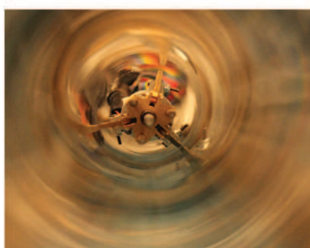
(B) Side view of the robot inside the pipe
