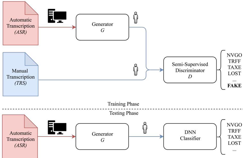
Figure 1: Illustration of the M2H-GAN architecture at training (top) and testing (bottom) time. Red and blue lines show the ASR and TRS representation signal. Note that the output of the generator  $G$  goes from red to blue during the training phase.
