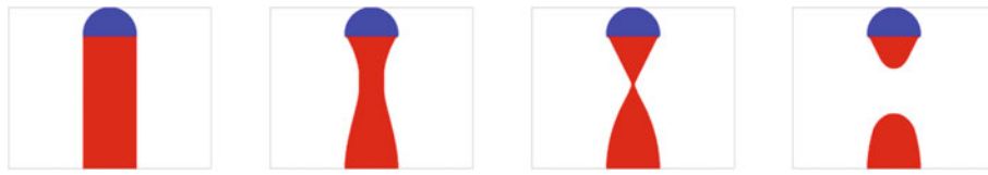
Fig. 8. Evaporation sequence of a bilayer structure. The field ratio at the interface is 2.5. The low evaporation field red layer is evaporating while the blue layer is not, eventually resulting in a fracture of the tip.
