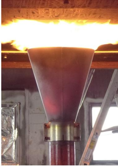
Figure 1: Picture of a running Park DPL 3400 kerosene burner
