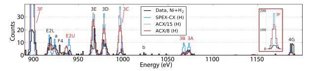
Figure 3: Laboratory measurements of CX with  $H_2$  on Ni L-shell ions compared with models, from [59]. Wide discrepancies exist between models and data, especially for the weaker lines.
