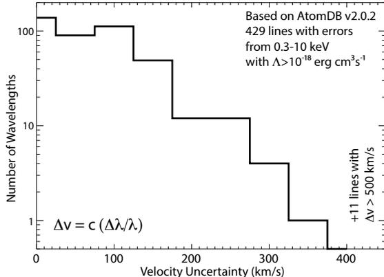
Figure 2: *Histogram of wavelength uncertainties for the strongest lines in the AtomDB v2.0.2 database. More than half have errors that will dominate the measured values from XRISM and Athena. From [28].*
