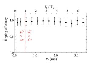
FIG. 4. (Color online) Flipping efficiency as a function of flipping time. The sweeping range  $\Delta_0$  and the Rabi frequency of the rf field are kept constant. The flipping efficiency is measured for different values of the chirp rate r. The flipping time  $\tau_f$  varies from a small fraction of  $T_2$  to more than 6 times  $T_2$ .
