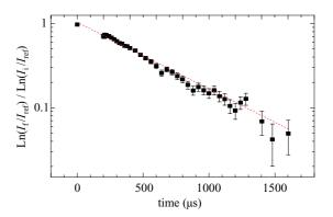
FIG. 2. (Color online) Decay of the optical transmission at the end of the spin refocusing sequence as a function of  $2(\tau_1 + \tau_2)$  (see Fig. 1). The exponential decay fit (red dashed line) leads to  $T_2 = 550 \pm 12 \ \mu s$ .
