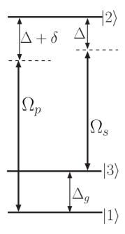
FIG. 1. Three-level  $\Lambda$  system where the ground-state hyperfine levels are split by  $\Delta_g$ . The optical, or one-photon, detuning is labeled  $\Delta$  and is the frequency difference between the Stokes pulse and the transition  $|3\rangle-|2\rangle$ . The two-photon detuning  $\delta$  is the detuning from resonant two-photon excitation of Raman transition. The Rabi frequencies of the pump and Stokes pulses are labeled  $\Omega_p$  and  $\Omega_s$ , respectively.
