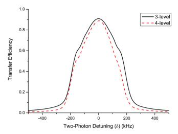
FIG. 5. (Color online) Two-photon detuning scan at optical resonance  $\Delta$ =0. The solid line (black) is the simulation of the standard three-level model and the dashed line (red) is the result from the four-level model. In these models the Rabi frequency on the strong transition was 400 kHz, the ground-state splitting was 7.1 MHz, the excited-state splitting was 2.84 MHz, and the pulse delay was -17  $\mu$ s.
