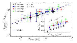
FIG. 3. Mean amplitude of the microscopic stick-slip  $A_{mss}$  as a function of the mean duration  $T_{mss}$  for peel experiments at L = 1 m and  $\theta = 90^{\circ}$ , with tape of different ribbon thicknesses measured in numbers of superimposed glued backings.
