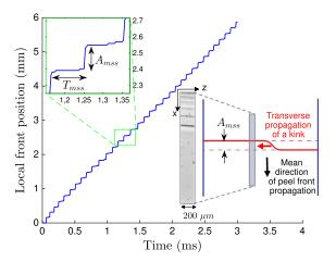
FIG. 1. Micro-stick-slip dynamics of the local longitudinal position of the peel front during an experiment at V = 1.8 m/s, L = 50 cm, and  $\theta = 90^{\circ}$ , with periods of rests  $T_{\rm mss}$  preceding slips of size  $A_{\rm mss}$ , as a result of the transverse propagation across the tape of a kinked fracture of amplitude  $A_{\rm mss}$ . We also display a typical image recorded by the fast camera (the gray zone in the inset gives its reduced field of view).
