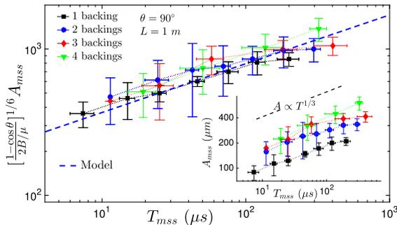
FIG. 3. Mean amplitude of the microscopic stick-slip  $A_{\text{mss}}$  as a function of the mean duration  $T_{\text{mss}}$  for peel experiments at  $L = 1 \text{ m}$  and  $\theta = 90^\circ$ , with tape of different ribbon thicknesses measured in numbers of superimposed glued backings.
