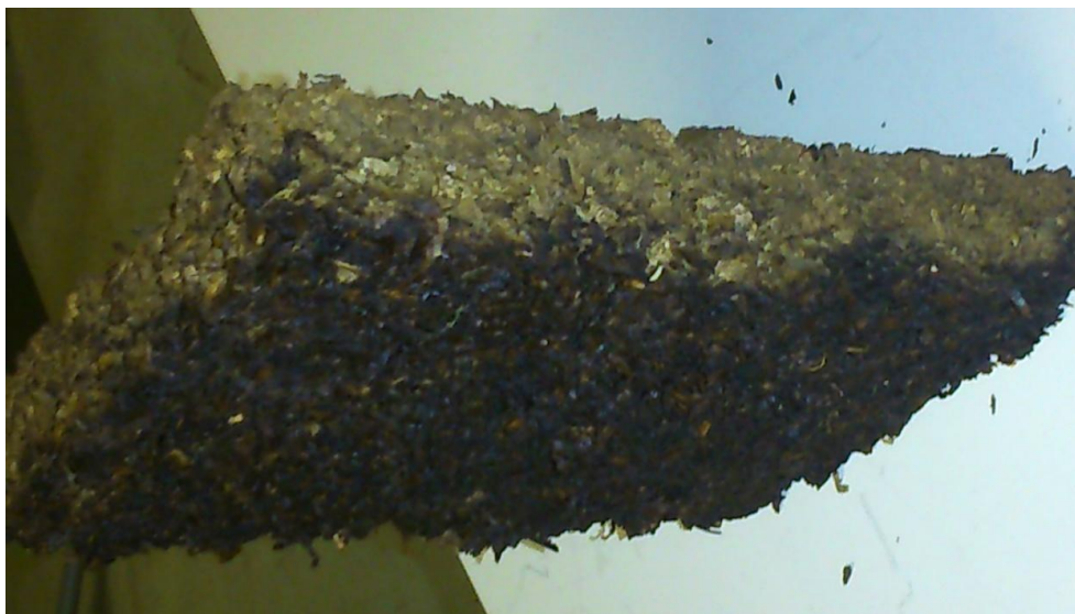
Figure 7. Impregnated sawdust at the end of the drying operation.
