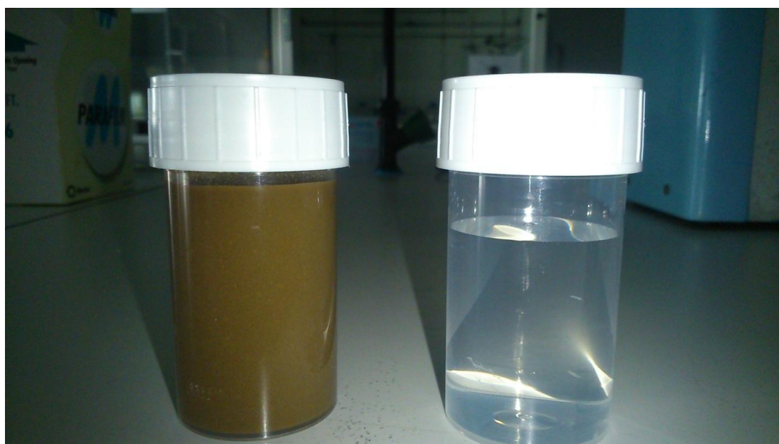
Figure 8. Aspect of OMWW (left) and recovered-condensed water from raw OMWW (right).
