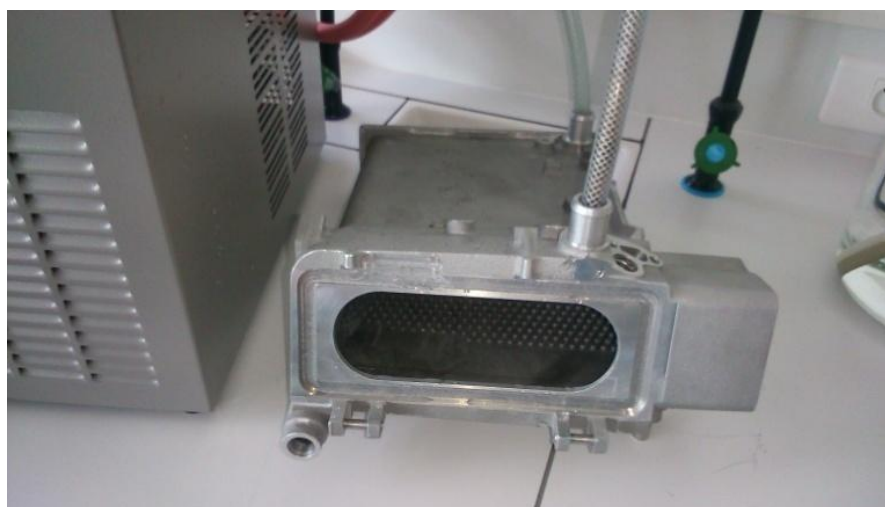
Figure 3. Boiler condenser used for the water recovery experiments.
