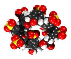
Figure 3. Self-Inclusion of one of the sulphonate group of C8S in complex 1.
