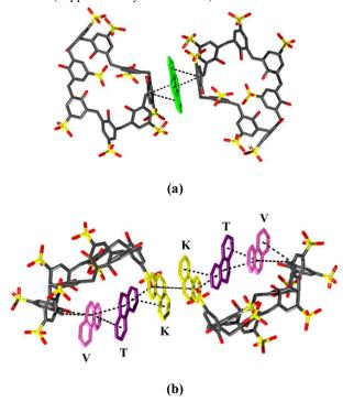
Figure 5. Phen cations intercalated between two adjacent C8S anions; (a) intercalation of a single cation Phen J (b) intercalation of Phen<sub>6</sub> hexamer (Phen cations are disordered, only one orientation of cations V/M, T/L and K/Q is shown for clarity).
