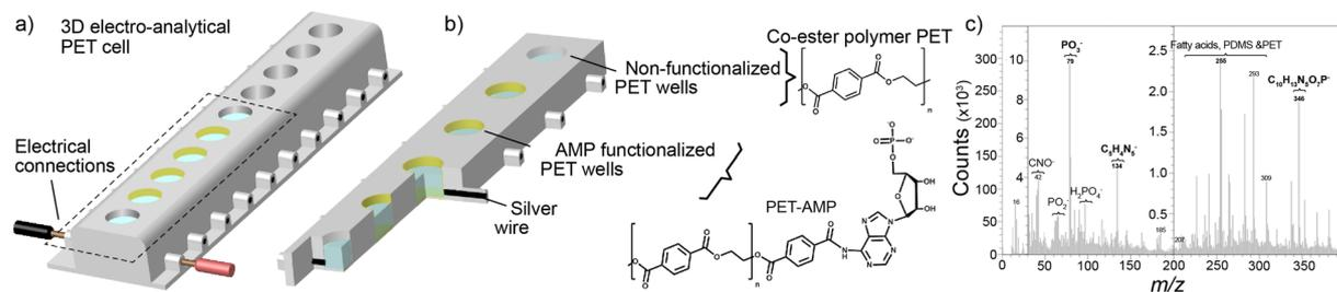
**Figure 5.** (a) Schematic representation of 3D printed PET electro-analytical cells for resistivity measurements. (b) The wells are filled with a solution (blue) to measure resistivity for AMP functionalized wells (orange/yellow) and non-treated wells (grey). Lateral inlets are filled with silver to measure the resistivity at the interface polymer/solution by multimeter probes (in black and red). (c) The ToF-SIMS spectra after surface functionalization.
