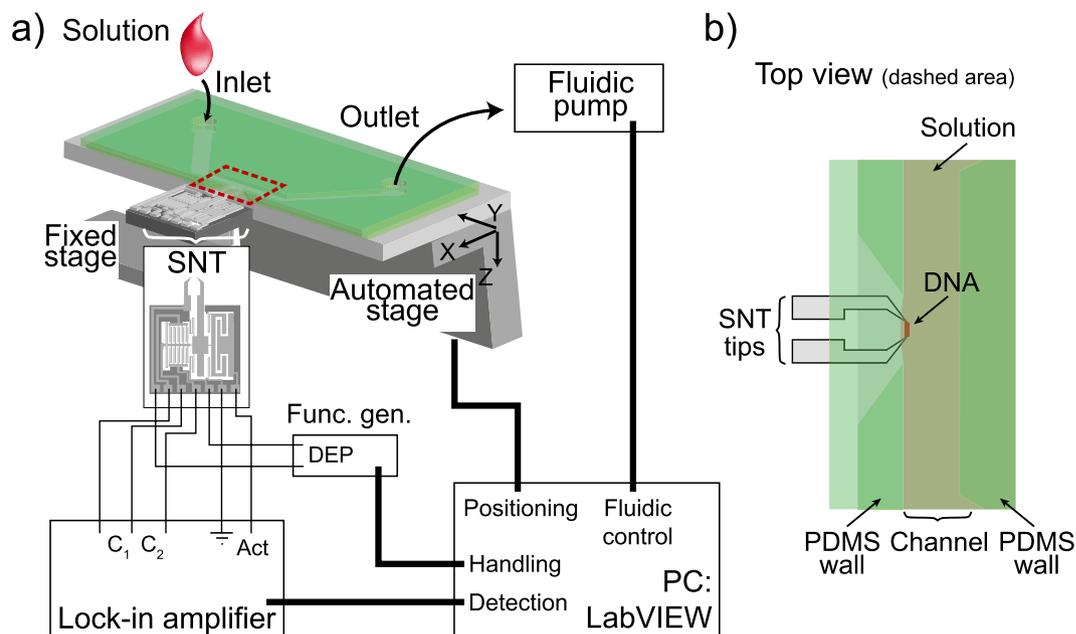
**Figure 2.** (a) The SNT device setup. (b) Immersion of the SNT tips in the channel of the microfluidic device, allowing the captured DNA bundle to interact with different solutions without passing through the meniscus, and hence avoiding strong mechanical stress on the bound DNA bundles.
