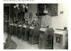
equipped with a binocular optic. Here, no film, but a hub on which the images are plugged. The fast rotation on the hub restores the animation.
