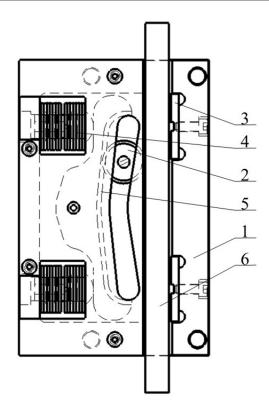
**Figure 1** Schematic representation of the CHP 2000 safety gear used by a friction crane brake system, which consists of the following parts: 1 - steel body; 2 - brake roller; 3 - thrust plate; 4 - spring package; 5 - braking cam; 6 - lift guide.
