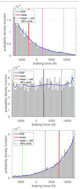
Figure 11 Probability density functions and statistical measures for the braking force with different input mean values for  $F_s$ : 14 kN (top); 28 kN (middle); 42 kN (bottom).
