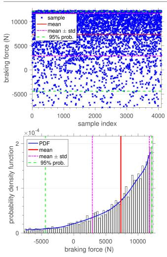
Figure 8 Generated samples (top) and probability density function (bottom), with statistical measures, for the braking force.
