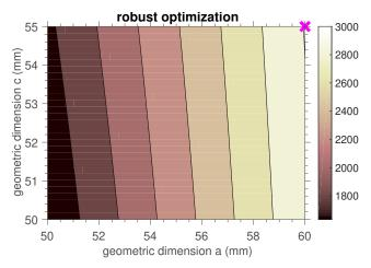
Figure 14 Contour map for the robust objective function with the optimum point is indicated by a cross.
