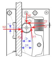
Figure 5 Illustration of the forces (in red) acting on the brake roller inside the safety gear and and the underlying geometric dimensions (in blue).
