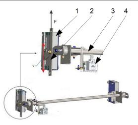
**Figure 2** Illustration of a typical friction crane brake system used by lifting devices, which consists of the following parts: 1 - safety gear cabin; 2 - trigger lever; 3 - safety gears connector; 4 - rope speed limiter.
