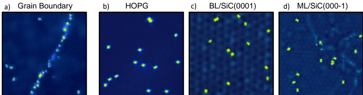
**Figure 4.** a) STM image of a graphene grain boundary heavily populated by hydrogen atoms. (b-d) STM images after the atomic hydrogenation of graphene layers on different substrates. All (b-d) images, with sizes of 20x20 nm<sup>2</sup> and hydrogen concentrations of ~0.17%, show most H atoms forming O and P dimers. Hydrogenation was performed at 140K in all cases.
