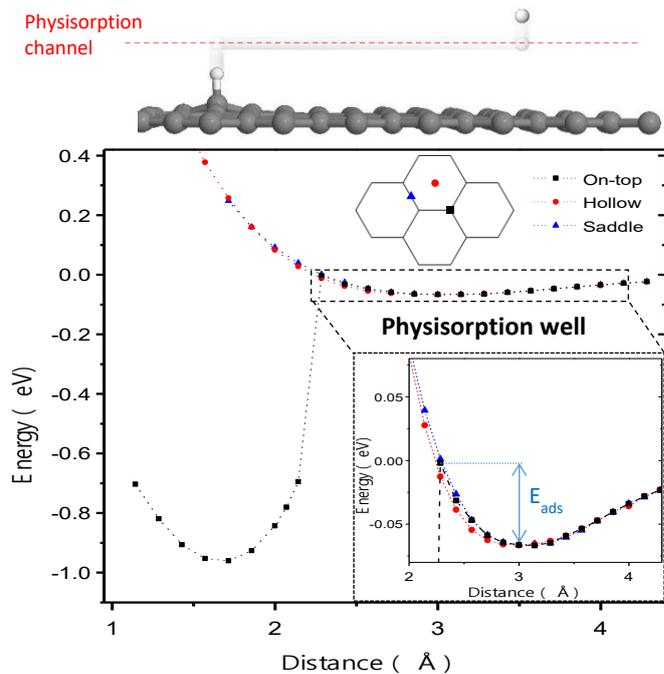
**Figure 2.** Energy-distance curves of the adsorption of a single hydrogen atom on 3 different positions of the graphene lattice: on-top, hollow and saddle. The energy is referred to the case of hydrogen and graphene being far apart. Inset: zoom in of the physisorption well. Upper drawing illustrates the adsorption path followed by a hydrogen atom towards the chemisorption state.
