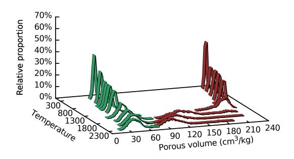
**Figure 5.** Comparison of temperature-dependent porosity between ZIF-4 (green) and ZIF-8 (red). The relative stability of the porous volume in ZIF-4 is striking compared to the collapse of the one in ZIF-8.
