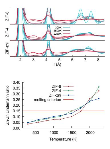
**Figure 1.** Top panel: Radial distribution functions for the pair of zinc and nitrogen atoms in the three ZIFs as a function of temperature. Bottom panel: Comparison of the evolution of the Lindemann ratios for the 3 ZIFs showing melting is happening at different temperatures.
