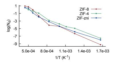
**Figure 3.** Top panel: Distribution of discrete zinc-nitrogen coordination numbers as a function of temperature for ZIF-8, ZIF-4 and ZIF-zni. Bottom panel: van 't Hoff plot of the number of defects. The formation of defects follows an Arrhenius law with respective activation energies of 59, 52 and 50 kJ.mol<sup>-1</sup> for ZIF-8, ZIF-4 and ZIF-zni.
