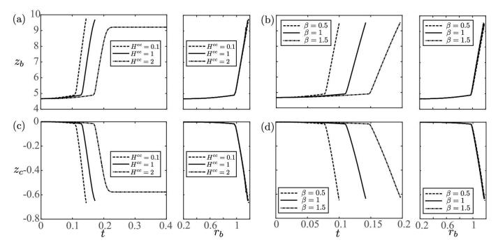
FIG. 4: Influence of the physico-chemical parameters for  $\theta = 2^{\circ}$ . Evolution in time of (a,b) the bubble position  $z_b(t)$  and (c,d) the cone position  $z_c(t)$  for different values of (a,c)  $H^{cc}$  and (b,d)  $\beta$ . In (a,c)  $\beta = 1$  and in (b,d)  $H^{cc} = 0.1$ . In each panel, the figure on the right show the evolution of  $z_b$  or  $z_c$  with respect to  $r_b$ .
