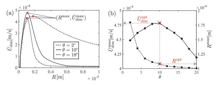
FIG. 7: Optimal microrocket design: (a) Evolution of the average dimensional velocity with the cone radius around the reference conditions for different opening angles. (b) Evolution with cone opening angle  $\theta$  of the average velocity,  $\bar{U}_{\text{dim}}^{\text{max}}$ , and corresponding cone radius at which the maximum is attained,  $R^{\text{max}}$ .
