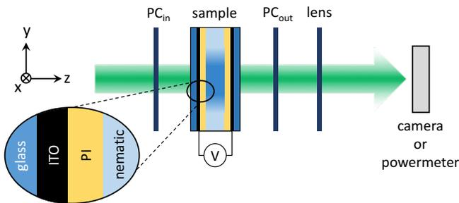
FIG. 1. Sketch of the experimental setup.  $PC_{in/out}$ : input/output polarization controllers. The lens is placed to image either the sample plane (using 75 mm focal length) or the far-field via optical Fourier transform (using 150 mm focal length) onto the camera.
