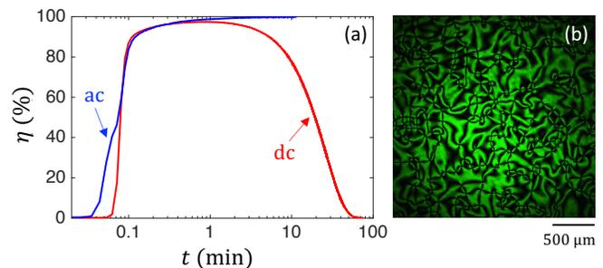
FIG. 3. (a) Polarization conversion dynamics at  $V = V_{\pi}$  for ac (blue curve) and dc (red curve) situations. Incident beam parameters: waist radius is 1.3 mm and total power is 0.25 mW. (b) Typical random network of umbilical defects with topological charge  $\pm 1$  imaged between crossed linear polarizers 30 s after the voltage is switched on at time  $t = 0$ .
