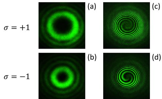
FIG. 5. (a,b) Total far-field intensity profiles of the self-induced steady-state optical vortex beams generated at  $V = V_\pi$  in the dc case under total incident power  $P = 10 \text{ mW}$ , incident beam waist radius  $w = 260 \mu\text{m}$ , and incident helicity  $\sigma = \pm 1$ . (c,d) Spiraling interference patterns obtained by superposing the output beam with a coherent coaxial Gaussian reference beam.
