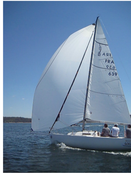
(b) "Optimal trim", periodic flapping of the leading edge.
