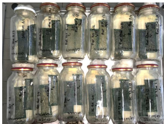
Fig. 3 : Samples in contact with fungal decay.
