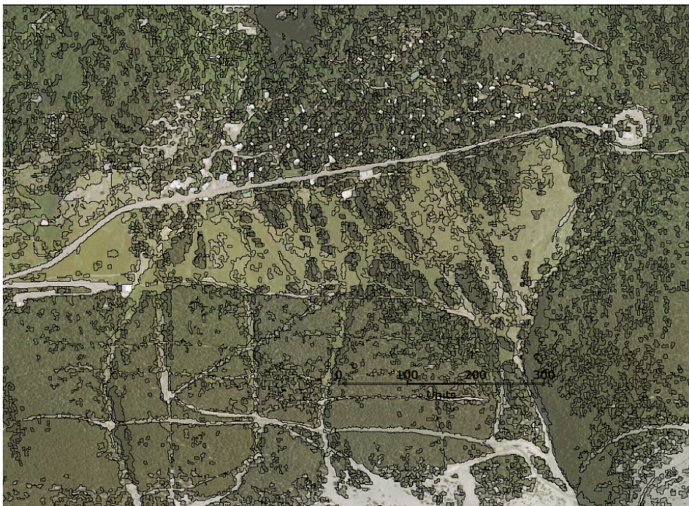
Figure 6. Segmentation obtained using Self Organizing Map (SOM-2-2-15) with the following parameters: radius = 2, alpha = 2 and K = 15 [39].
