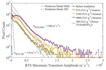
Fig. 7. Distributions of the PPDs RTS maximum transition amplitude of the leakage current before and after 50-MeV protons and 22-MeV neutrons irradiations.
