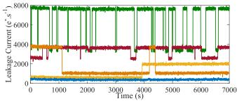
Fig. 6. Leakage current evolution with time of five FDs before irradiation. Four of them are exhibiting a leakage current RTS behavior.
