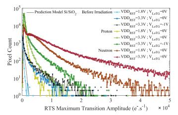
Fig. 12. FD leakage current RTS maximum transition amplitude distributions for several biasing conditions before and after neutron (DDD =  $40\,000$  TeV  $\cdot$  g<sup>-1</sup>) and proton [DDD = 500 TeV  $\cdot$  g<sup>-1</sup> and TID = 24 krad(SiO<sub>2</sub>)] irradiations.
