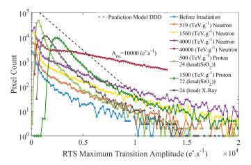
Fig. 8. Distributions of the FDs RTS maximum transition amplitude of the leakage current before and after 50-MeV protons and 22-MeV neutrons irradiations. The slope of the prediction model is at  $A_{\text{rts}} = 1200 \text{ e}^{-1} \cdot \text{s}^{-1}$ .
