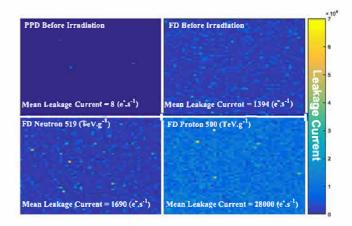
Fig. 2. Image depicting the leakage current in the PPDs before irradiation and in the FDs before and after irradiation.
