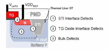
Fig. 10. Cross section of the FD structure showing the different leakage current sources.
