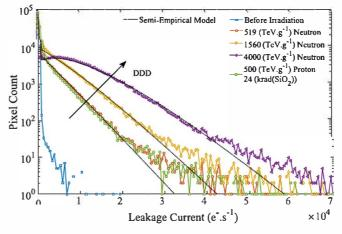
Fig. 4. Distributions of the PPDs leakage current after 50-MeV protons and 22-MeV neutrons irradiations.
