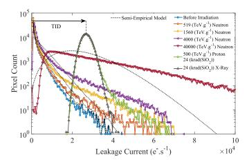
Fig. 5. Distributions of the FDs leakage current after 50-MeV protons and 22-MeV neutrons irradiations.
