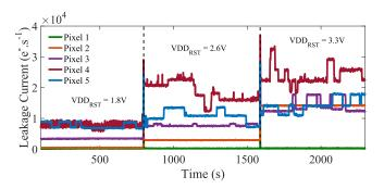
Fig. 14. FD leakage current evolution with the reset voltage after proton irradiation 500 TeV  $\cdot$  g<sup>-1</sup> and 24 krad(SiO<sub>2</sub>).
