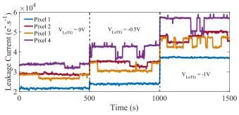
Fig. 13. FD leakage current evolution with the TG bias after proton irradiation 500 TeV  $\cdot$  g<sup>-1</sup> and 24 krad(SiO<sub>2</sub>).
