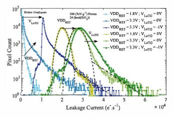
Fig. 11. FD leakage current distributions for several biasing conditions before and after proton irradiation DDD =  $500 \text{ TeV} \cdot \text{g}^{-1}$  and TID =  $24 \text{ krad}(\text{SiO}_2)$ .
