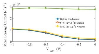
Fig. 9. Evolution of the FD leakage current with TG OFF-voltage before and after 50-MeV protons and 22-MeV neutrons irradiations.
