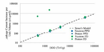
Fig. 3. Evolution of the mean leakage current increase per unit volume with irradiations. The considered UDF value after one month annealing is  $K_{\text{dark}} = 0.098 \text{ e}^{-1} \text{ s}^{-1}/\text{Tev} \text{ s}^{-1}/\mu\text{m}^3$  [13].
