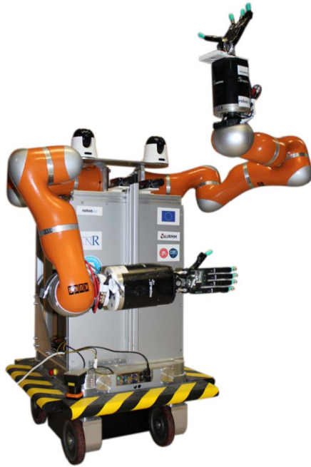
Fig. 1 The BAZAR (Bimanual Agile Zany Anthorpomorphic Robot) collaborative robot designed at LIRMM. The platform includes: one Neobotix MPO 700 omni-directional mobile base with two Hokuyo UTM-30LX laser scanners, one Microsoft Kinect V2 RGBD camera (not show in this figure), two AVT Prosilica GT Gige/PoE RGB cameras, two DLINK DCS 5222L pan-tilt RGB cameras and two KUKA LWR4+ arms. Each arm is equipped with one ATI Mini 45 force/torque sensor, one Shadow Dexterous Hand with SynTouch LLC Biotac tactile sensors and a Leapmotion vision sensor mounted on the hand wrist.
