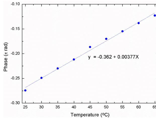
Figure 5. Optical sensor’s response towards temperature variations.
