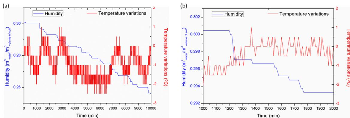
Figure 6. (a) Temperature and humidity measured during a week in Soil1 and (b) a detailed region.
