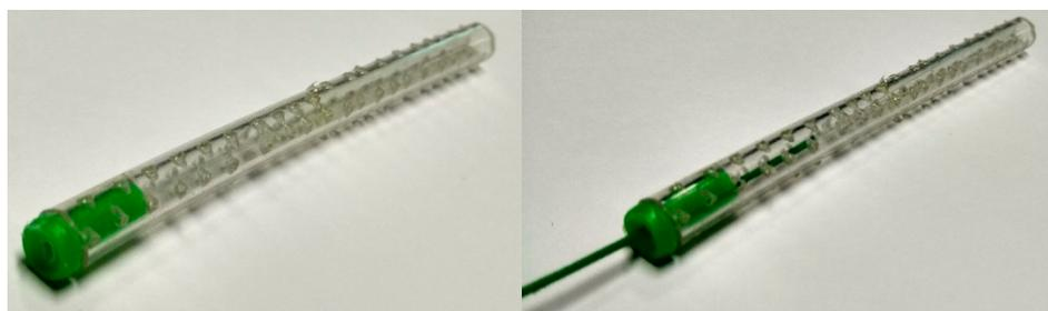
**Figure 2.** Optical sensor's polyvinylchloride (PVC) drilled protective cap.
