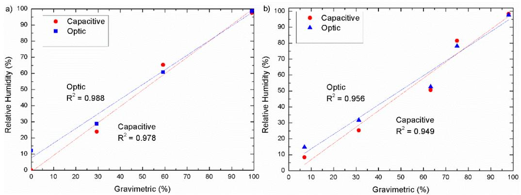
Figure 9. Capacitive and optical sensor’s regression slopes: (a) Soil1 and (b) Soil2.
