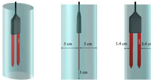
Figure 10. Idealized measurement volume of Decagon 10HS sensor.
