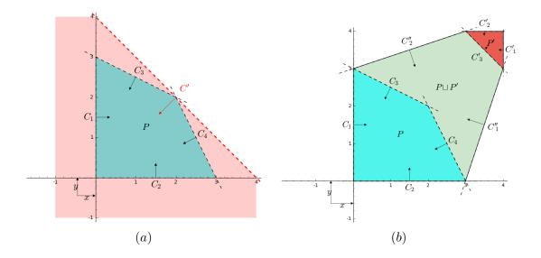
Figure 1: Representation of polyhedron  $P: \{C_1: x \geq 0, C_2: y \geq 0, C_3: x+2y \leq 6, C_4: 2x+y \leq 6\}.$ (a): Constraint  $C': x+y \leq 4$  includes P, because  $C'=\frac{1}{5}C_2+\frac{1}{5}C_4$ .
