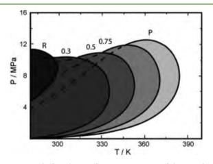
**Figure 5.** Hydroformylation of propene: progress of the two-phase boundary for a six-component reaction mixture, as the reaction proceeds through different conversions: R (reactants), 0.3, 0.5, 0.75, and P (products), indicated in the figure, as calculated by Ke et al.<sup>90</sup> Reprinted with permission from Nunes da Ponte, M. *J. Supercrit. Fluids*, **2009**, 47 (3), 344–350. Copyright 2009, Elsevier.
