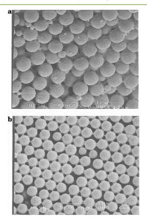
**Figure 4.** Scanning electron micrographs for particles formed (a) without  $CO_2$  and (b) with  $CO_2$  at 113 bar. Both samples are taken at about 80% of conversion. Reprinted with permission from Quadir, M. A; Snook, R; Gilbert, R. G.; DeSimone, J. M. *Macromolecules* **1997**, 30 (20), 6015–6023. Copyright 1997, American Chemical Society.
