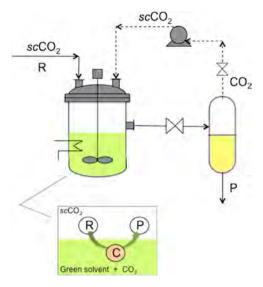
Figure 1. General schema showing a  $scCO_2$ /green solvent biphasic reactional system with R = reactants, P = products, and C = catalyst.
