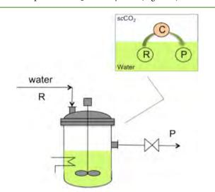
**Figure 3.** General schema showing an inverted  $scCO_2$ /water biphasic reactional system where  $scCO_2$  acts as a reservoir for the catalyst and water is the reactants and products carrier; R = reactants, P = products and C = catalyst.
