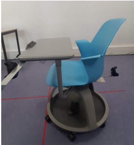
Figure 3: A mobile chair to be represented in the immersive environment, equipped with Vive trackers (one on the chair, one on the tablet).
