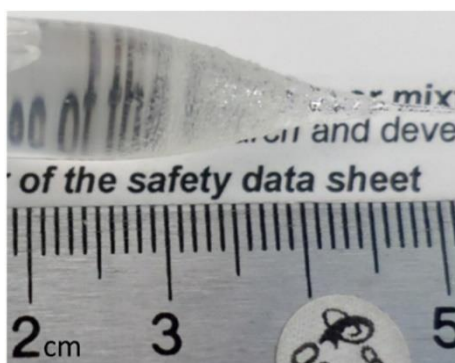
Fig. 13. Photograph of a GGBK17 preform neck-down after a conventional fiber drawing at 805 °C.
