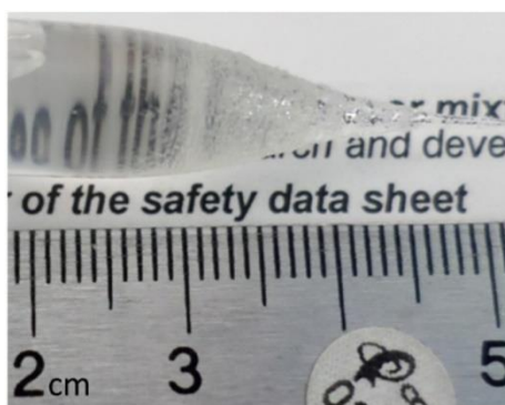
Fig. 13. Photograph of a GGBK17 preform neck-down after a conventional fiber drawing at 805 °C.
