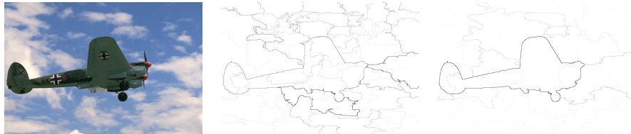
Fig. 1: Saliency maps resulting from the HGB method using the original observation scale (middle) and from one of our proposed observation scale (right).
