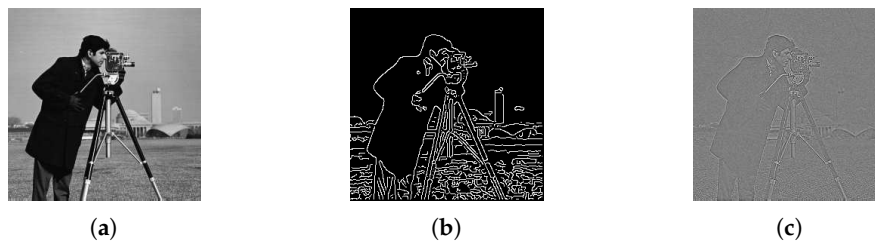
Figure 5. Image information at different levels. (a) Gray image. (b) Edge feature image. (c) Reconstructed image using phase angle.
