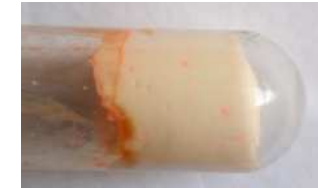
Gelled emulsions : Network of proteins entrapping oil droplets
