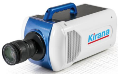
Kirana, uCMOS, 30 \mu m, 2Mfr/s, 180 images, 924*768pixels 416x228x192mm, 10.5kg
