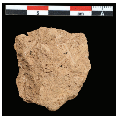
Fig. 4. Mud-brick 35087_Bot1. Detail of the plant temper. Imprints of date palm leaves (arrows).
