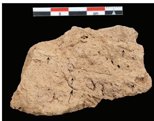
Fig. 3. Mud-brick 35087_Bot1. Detail of the plant temper. Imprints of cereal grains (long arrow) and stems (short arrows).
