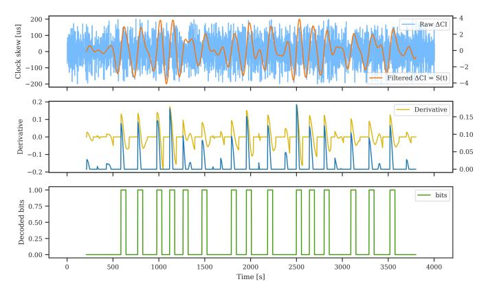
Figure 9: Covert channel on the iPhone 5s. No temperature information was easily available, so the heat graph is omitted.
