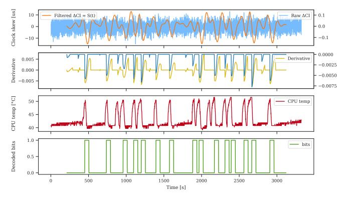
Figure 7: Covert Channel on the cooled Raspberry Pi. The cool down phase is quicker then the heat up phase. We search for strong negative spikes in the filtered clock skew signal instead of positive spikes.
