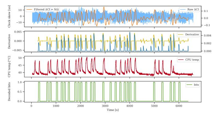
Figure 4: Implementation of the covert channel on the Raspberry PI 3B. From top to bottom: raw and filtered skew, the derivative of the filtered skew, the CPU temperature and the decoded bits.
