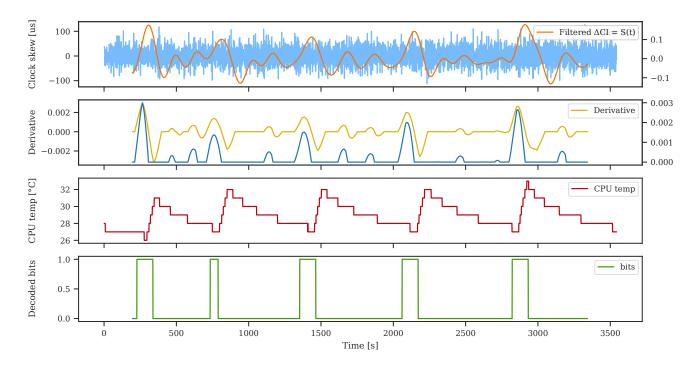
Figure 8: Covert channel on the Motorola X 2014. Compared to the filter clock skew on the Raspberry Pi platform, the clock skew variations are much more suppressed.
