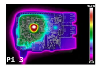
Figure 6: Thermal image of the RPi 3B (source: [13]).
