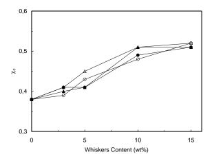
Figure 11: Evolution of the degree of crystallinity of the LDPE matrix as a function of the ramie cellulose whiskers content for nanocomposite films reinforced with unmodified ( $\bullet$ ) and modified with hexanoyl chloride ( $\circ$ ), lauroyl chloride ( $\triangle$ ) and stearoyl chloride ( $\Delta$ ) whiskers. The lines serve to guide the eyes.
