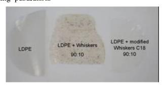
**Figure 10:** Photographs of the neat film and ramie cellulose whiskers based nanocomposite films reinforced with 10 wt% of WRU and WRC18.
