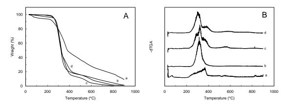
**Figure 8:** TGA curves (A) and dTGA (B) for unmodified ramie cellulose whiskers (a) and modified with hexanoyl chloride (b), lauroyl chloride (c) and stearoyl chloride
