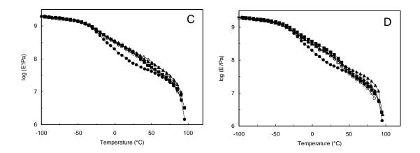
**Figure 12:** Evolution of the logarithm of the storage tensile modulus as a function of temperature for the neat LDPE matrix (●) and related nanocomposite films reinforced with 3 (A), 5 (B), 10 (C) and 15 wt% ramie cellulose whiskers: unmodified (○) and modified with hexanoyl chloride (▲), lauroyl chloride (△) and stearoyl chloride (■).
