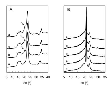
**Figure 6:** Wide-angle X-ray diffraction patterns for ramie cellulose whiskers (A): unmodified (a) and modified with hexanoyl chloride (b), lauroyl chloride (c) and stearoyl chloride (d), and nanocomposite films (B): neat LDPE matrix (a) and related nanocomposite films reinforced with 10 wt% ramie cellulose whiskers: unmodified (b) and modified with hexanoyl chloride (c), lauroyl chloride (d) and stearoyl chloride (e).
