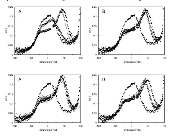
**Figure 13:** Evolution of the tangent of the loss angle  $(\tan \delta)$  as a function of temperature for the neat LDPE matrix ( $\bullet$ ) and related nanocomposite films reinforced with 3 (A), 5 (B), 10 (C) and 15 wt% ramie cellulose whiskers: unmodified ( $\circ$ ) and modified with hexanoyl chloride ( $\triangle$ ), lauroyl chloride ( $\Delta$ ) and stearoyl chloride ( $\blacksquare$ ).
