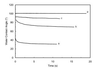
**Figure 7:** Water contact angle with time for unmodified ramie cellulose whiskers (a) and modified with hexanoyl chloride (b), lauroyl chloride (c) and stearoyl chloride (d).
