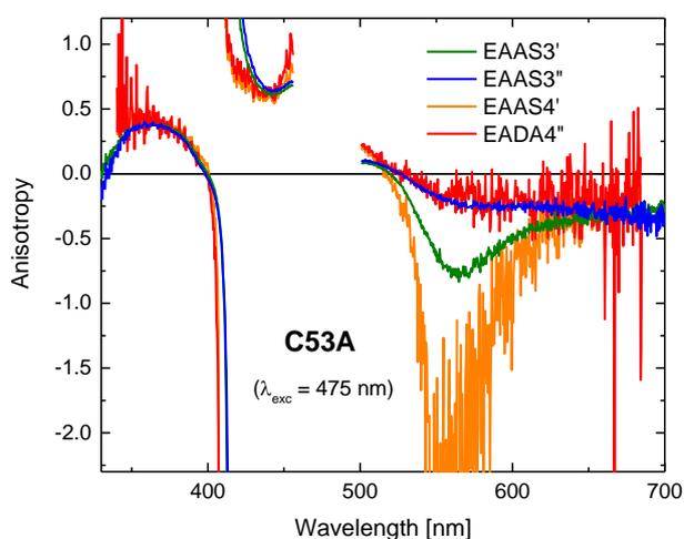
**Figure 5.** Correction of EAAS3 and EAAS4 in the case of C53A with excitation at 475 nm. EAAS' are the anisotropy spectra deduced from the polarized EADS' (Equation 3); EAAS'' are further deduced from EADS'' (Equation 4).
