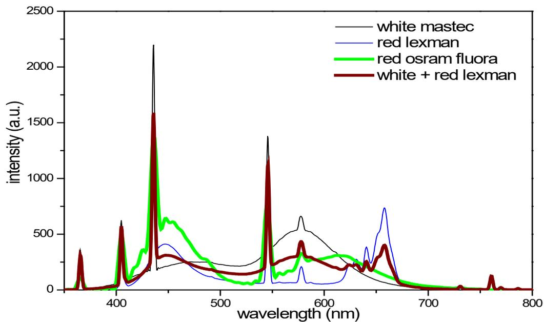
**Figure S1.** Light spectra of fluorescent lamps used for growth tests in low light. We used a mix of white (Mastec) and red (Lexman) lamps for test 1 and only Fluora lamps for test 2 and 3.
