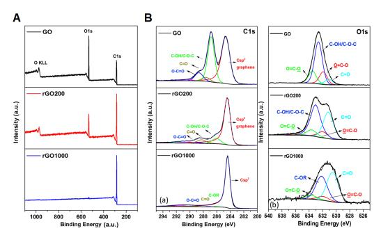
**Figure 2.** X-ray photoelectron spectroscopy (XPS) survey spectra of GO, rGO200 and rGO1000 materials (**A**); C1s and O1s deconvoluted XPS spectra for GO, rGO200 and rGO1000 (**B**).
