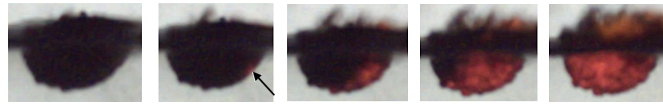
Figure 3: Apparition and propagation of an ignition flash ( T_{H_2O} = 52^\circ\text{C} ). Ignition appears locally and promptly extends to the whole gas film.
