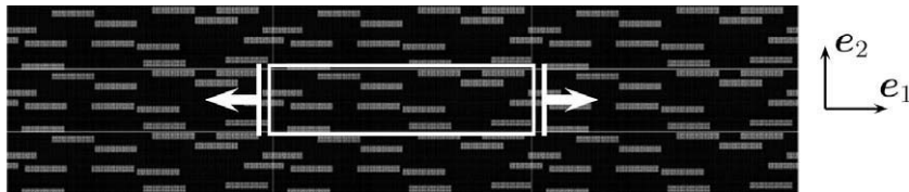
Fig. 5. Illustration of the chosen hydrided Zircaloy microstructure (20% of inclusions) reproduced by periodicity (nine RVEs).
