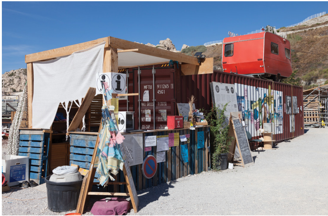
FIGURE 6 The campsite's reception desk. The reception desk of the campsite was built out of a recycled container (Photograph by Yes We Camp! 2013).
