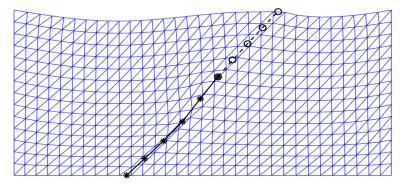
Fig. 3 Mesh sample of  $\Omega$  with real crack and fictitious crack (magnification=20)
