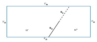
Fig. 1 Domain  $\Omega$  with the crack  $S_C$  and fictitious crack  $S_0$
