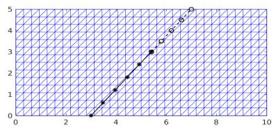
Fig. 2 Mesh sample of  $\Omega$  with real crack and fictitious crack
